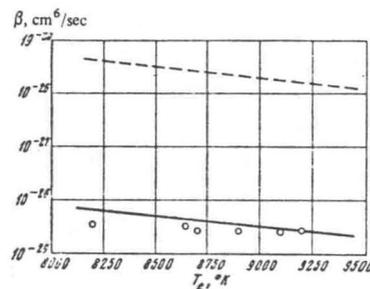
FIG. 8. Temperature dependence of the recombination rate constant of  $\text{Xe}^+$  in triple collisions: points—experimental values, solid curves—theoretical value [17], dashed—theoretical value [14].
